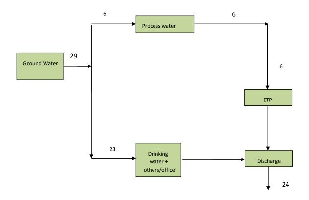
Figure 5: Water balance diagram
